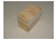
Cut 2x 2" chunks of a 2x4 and screw or glue them together (or you can use any 3" thick piece of wood that will fit into the hole you are going to make in the drywall).
